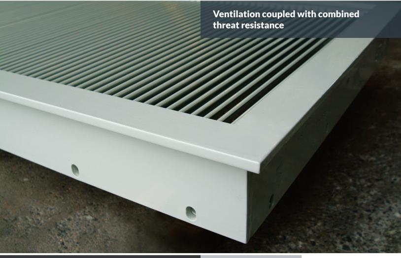
Maximum Security Louvers provide UL 752 and DOS-certified protection against mob-level forced-entry attacks and rifle-level ballistic threats in applications where buildings require airflow for equipment and occupants. A unique chevron slat design offers extraordinary protection against firearm assaults and exceptional rain shedding capabilities.
